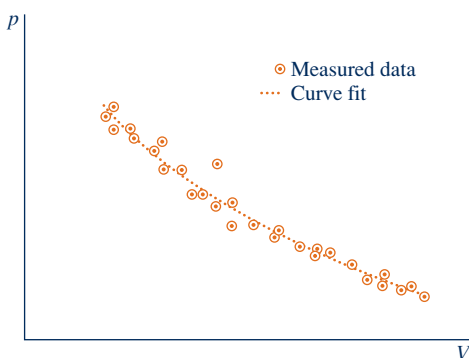
Fig. 2.5 Pressure at the piston face versus cylinder volume.
